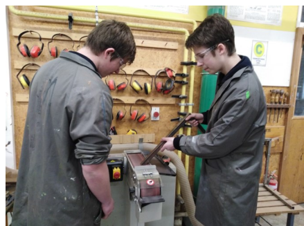
Left: Mathew Stephen and Zane Cochrane (both Year 12), using the Linisher to smooth off Zane's metal.
