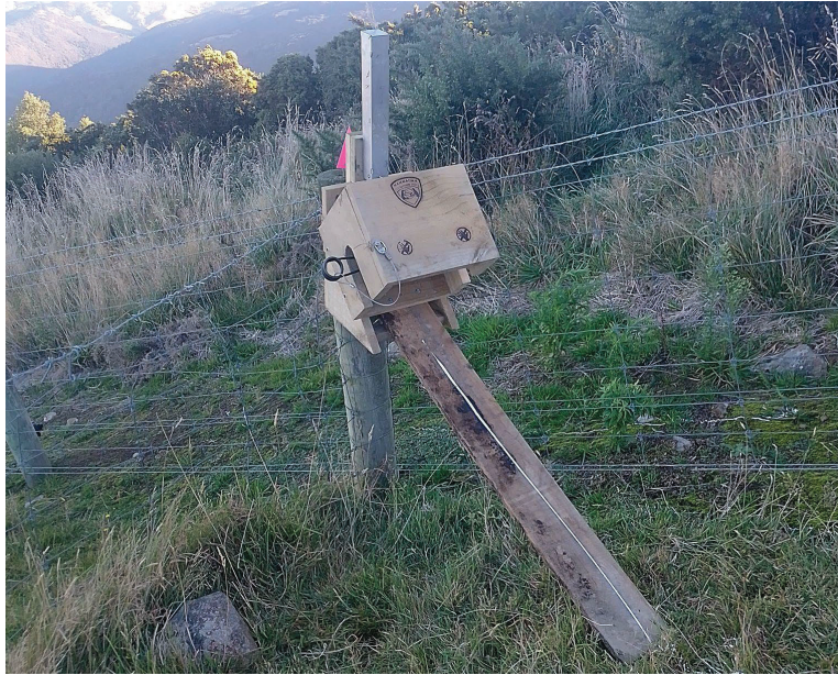
Image 3. Modified elevated prototype trap installed on a post using a 45° access ramp.
