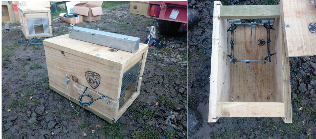
Image 6. Final enclosed SX220 trap design showing modified DOC250 trap box with removable entrance baffle and sliding end plate.
