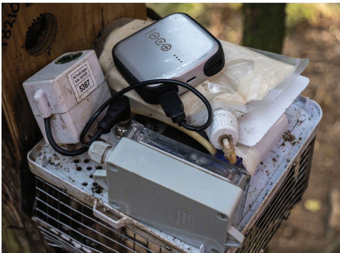
Figure 3. An audio lure (top center) placed inside the lid of the AT220. The device was programmed to play a territorial possum call at 15 min intervals each night. The battery capacity of the device allowed for 22 nights of playback.
