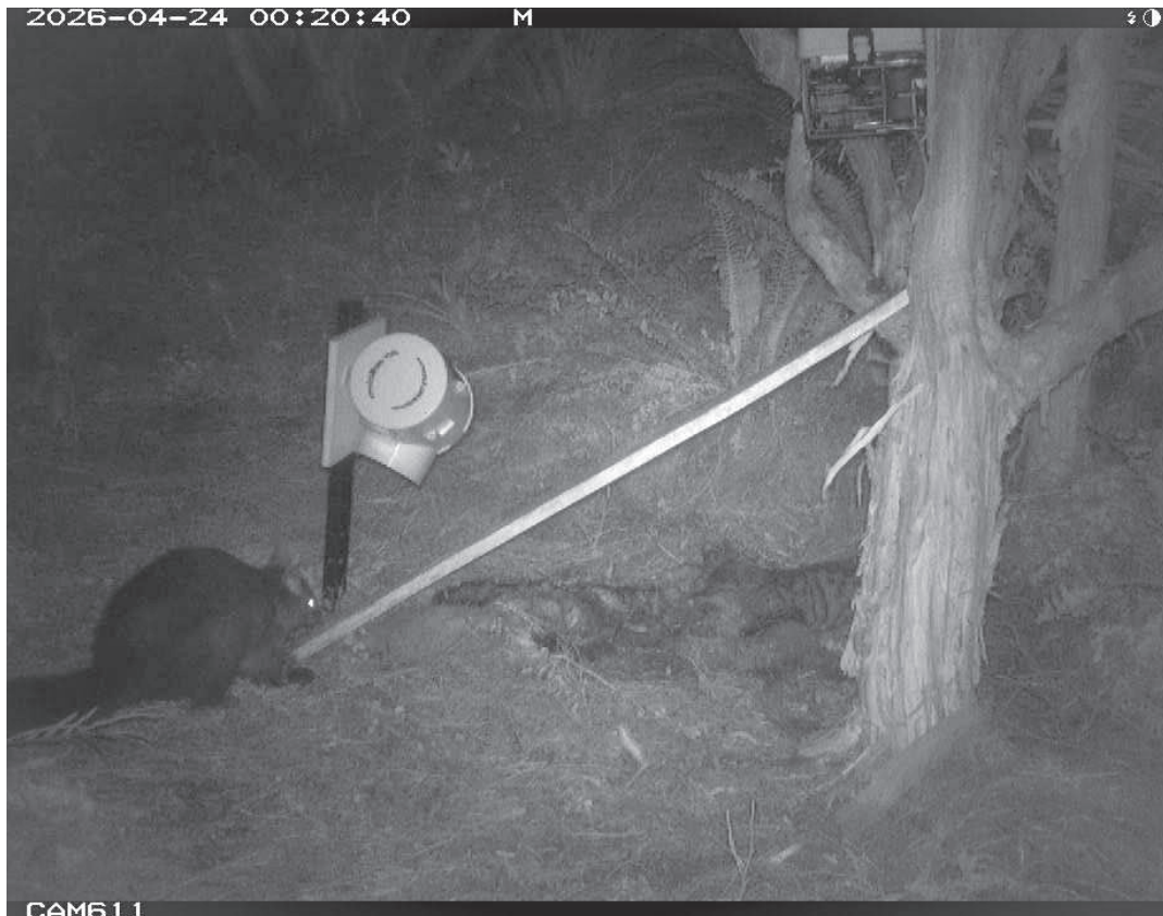
Figure 2. Possum investigating an oreo cookie that has been dispensed at the base of the AT220 trap ramp by an Enviromate bait dispenser. Pairs of cookies were dropped at 2-day intervals for 22 days.
