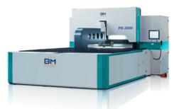
BM PB series is a new generation of fully automatic multilateral bending center. The product not only saves a lot of manpower, but the continuous bending speed is 3 times that of the CNC bending machine, reaching 0.2s/time.
