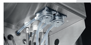
Concentrated cleaning: The metering pumps measure acid and alkaline cleaning agents automatically. A third metering pump can be used for disinfection.
