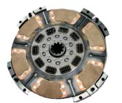
Eaton Easy Pedal 15" x 2" DCF 10 Spline Suits 1850 ft/lbs max torque
